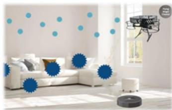
If you want to filter the air, you must go where the air is. That is the principle behind the ATAraina Flying Magic Cleaner. It is a drone that flies around your house like an airborne robot vacuum cleaner and filters your air. It uses a built-in ionizer to attract ultra-fine particles and run them through a filter. It has multiple cameras and sensors to avoid obstacles.
