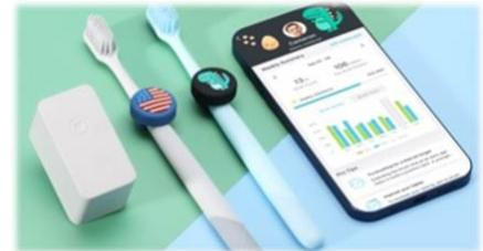
The tracker on the brush connects via Bluetooth to a plug-in hub that also supports Wi-Fi. Parents can monitor several brushes at once on the smart phone app to see the quality and time of brushing or get an alert if brushing hasn't occurred by a set time. No longer do you need to hover or interrogate when it comes to dental care.
