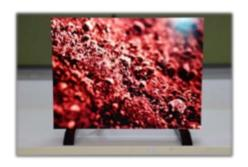
stacks the red, green and blue colors vertically and doesn't require wire bonding. This allows 2,000 color pixels per inch for amazing resolution. The current drawback is the price. While we don't have pricing for 2023, the 89-inch model from last year costs \$80,000 US. This year Samsung is offering a 50-inch model that will hopefully be much less expensive.
