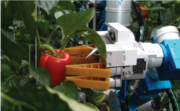
Researchers are testing robotic harvesting systems that use image recognition.
